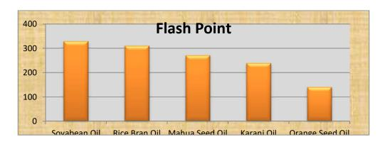
It is observed that Soyabean oil has highest flash point of 328°C followed by Rice bran oil which also has a flash point of 310°C. Orange seed oil, Mahua oil and Karanj oil seed oil had flash points of 140°C, 270°C and 239°C respectively.
