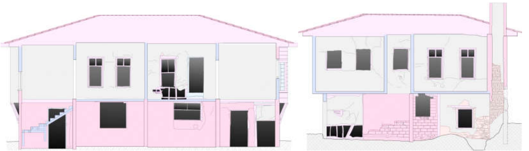
Figure 17. First Floor (Left) and First Floor Ceiling (Right) Damage Assessment Plan
