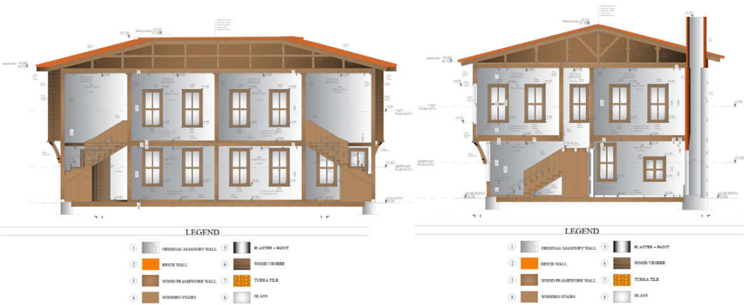
Figure 22. Building Section A–A (Left) and B–B (Right) – Restoration Project
