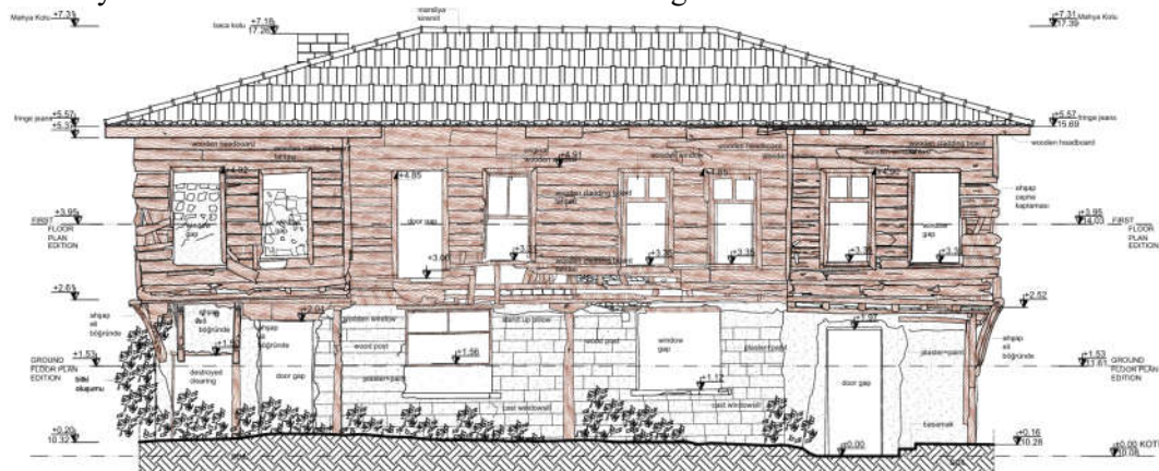
Figure 12. Eastern Facade Survey Drawing
