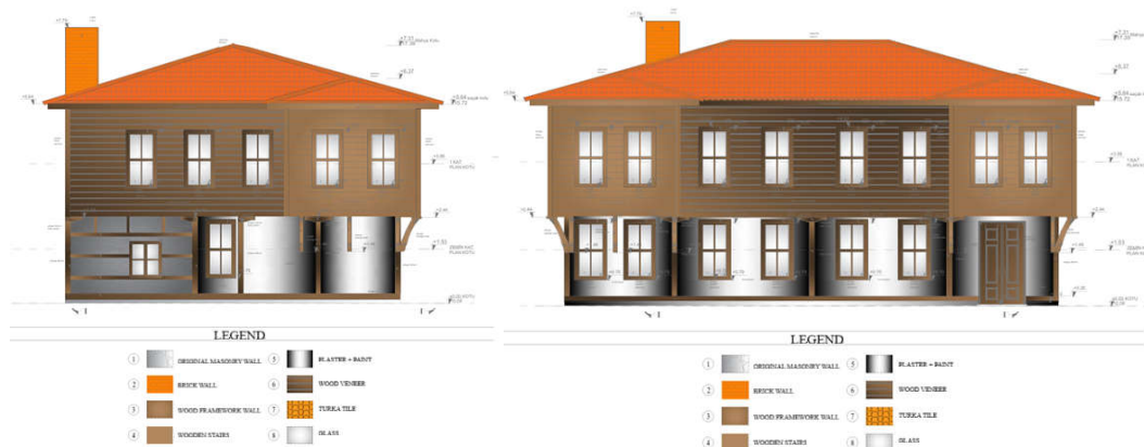
Figure 24. South (Left) and East (Right) Façade – Restoration Project
